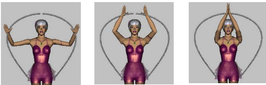
Fig. 2. A clapping exercise in our animation tool, where the movement path shown for the hands and the rotation of the wrists are defined by functions of time t , assigning a 3D point and a triple of Euler angles to each time moment of the entire duration
